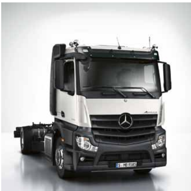
ClassicSpace cab, 2300 mm wide, engine tunnel 170 mm
